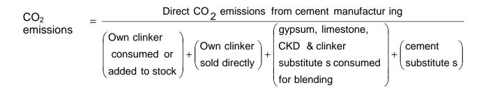
(2) CO<sub>2</sub> Emissions per metric tonne of Clinker
