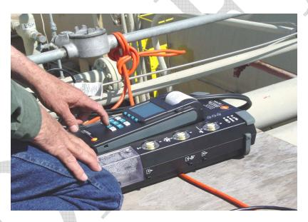
FOR THE PERIODIC MONITORING OF NITROGEN OXIDES, CARBON MONOXIDE, AND OXYGEN FROM STATIONARY ENGINES SUBJECT TO SOUTH COAST AIR QUALITY MANAGEMENT DISTRICT RULE 1110.2
