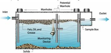
interceptor captures those wastes and contains them until a waste hauler or pumper service can properly dispose them. A grease interceptor should be checked and maintained to ensure that it is working properly. Backups, odors, and drainage problems are signs that the grease interceptor is not functioning as it should. See OCSD's Fact Sheet for Grease Interceptor for specific tips on proper maintenance of grease interceptors.
