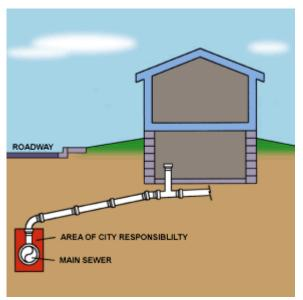
The side sewer, often referred to as a lateral sewer, carries your home's waste from toilets and drains to the City's main sewer line on its way to the wastewater treatment plant.
