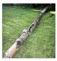
Deteriorated laterals on private property, such as the one pictured to the left, are an example of a private source of rainwater entering the sanitary sewer system.
