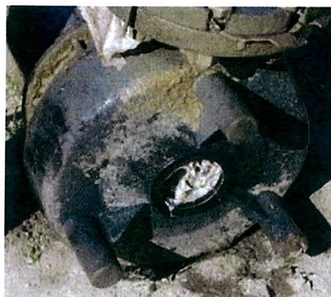
A Portland Water District (Maine) pump, clogged with wipes—an occurrence repeated across the country
