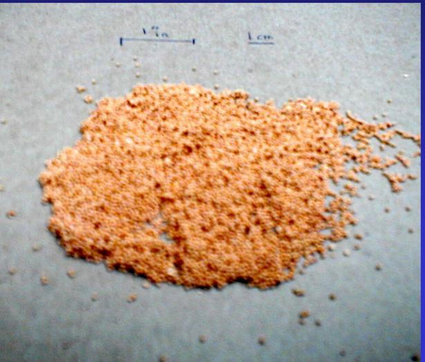
•Copolymer of Styrene/ Divinylbenzene •Hydrophobic •Low Affinity for Methane •Micropores 100-200 Angstroms
